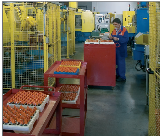
Loading the automated multi-axis CNC sharpening machines.
